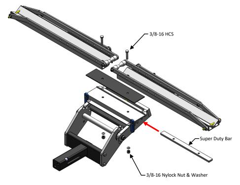
Note: Periodically tighten fasteners to insure secure connection.
