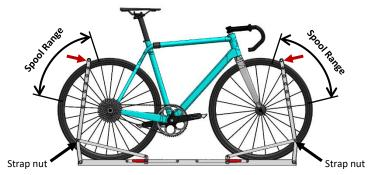
Note: Spool must contact tire within specified range. Bike is not secured in rack if spool is located outside of specified range.
