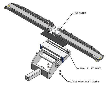
Note: Periodically tighten fasteners to insure secure connection.
